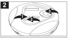
Within ten seconds, select the desired preset using the PRESET UP ▲ ① or DOWN ▼ ② button. Press the PROG button ③ to confirm.
