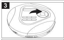
Press the PROG button to memorize the track. Repeat steps 2 and 3 to program additional tracks up to a maximum of 24 tracks.
