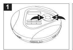
During playback, depress and hold either the Skip/TUNING ₩ ① or № ② button to move the player forward or backward within a track to locate a specific musical passage. The player will move forward or backward at high speed as long as the buttons are depressed. When you release the Skip/TUNING ₩ ① or № ② button, normal playback will resume.
