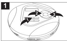
To repeat all files in a directory (MP3 CD only), press the MODE/◀ button ① three times; "REP D" will appear in the display. Press the Skip/TUNING № ② or № ② button to select the specific directory that you wish to repeat.
