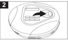
After you insert the disc into the CD player and the total number of tracks appear in the display, you may press either the Skip/TUNING M • or M • button to select a specific track for playback.
